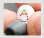
Try changing the the correct size foam tip. Do not use fingernail when removing the tip.
